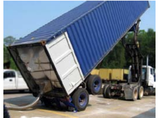
A lined shipping container is lifted for gravity flow.
