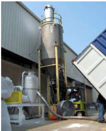
USS Vacuum/Pressure Conveyor transfers powder material to Bulk Bag Filling Station
